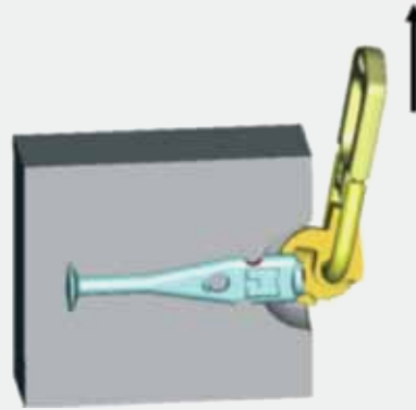
When pitching the concrete unit with the 3D Lifting System, the nose must be in the same direction with the load.
